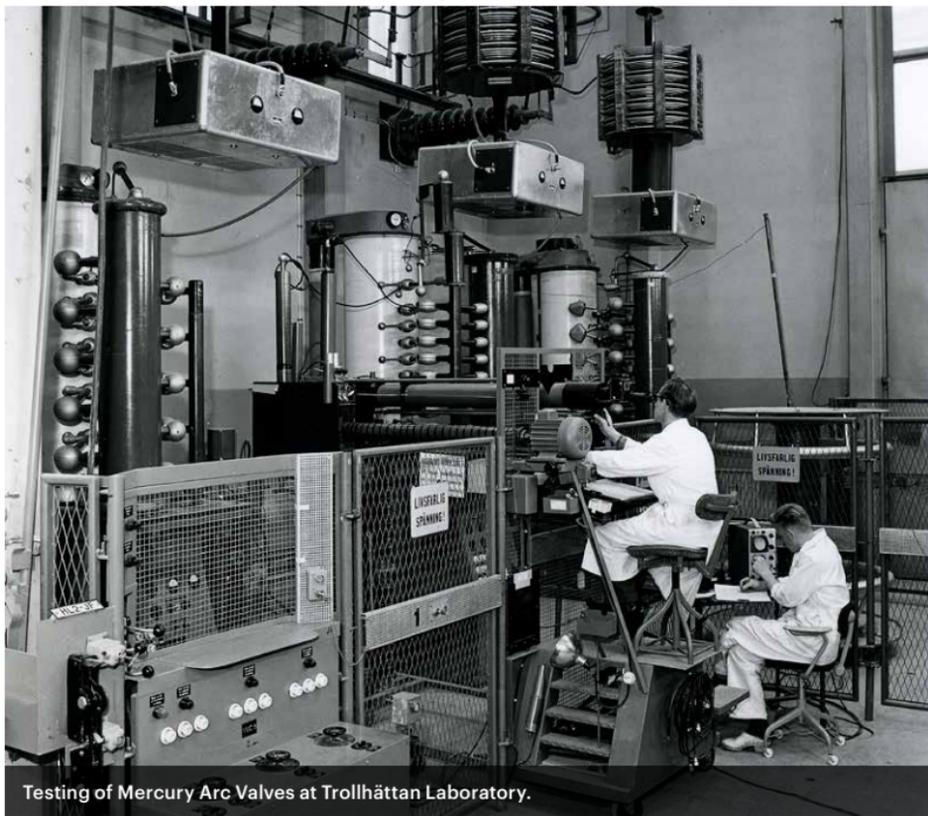
Testing of Mercury Arc Valves at Trollhättan Laboratory.
